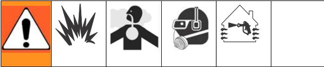
Spraying or dispensing materials containing isocyanates creates potentially harmful mists, vapors, and atomized particulates.
