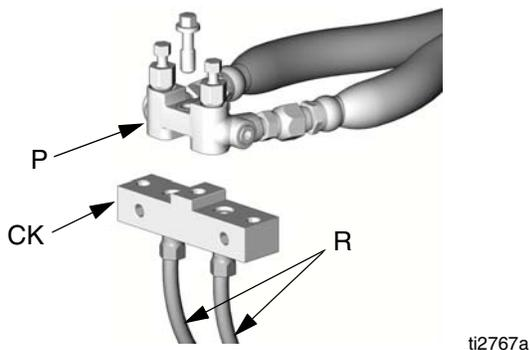
2. Route circulation lines back to respective component A or B supply drum. Use hoses
