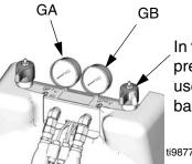
In this example, B side pressure is higher, so use the B side valve to balance pressures.
