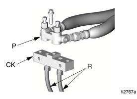
2. Route circulation lines back to respective component A or B supply drum. Use hoses
