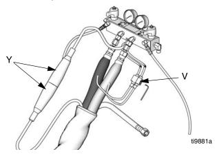
9. Close gun fluid manifold valves A and B
