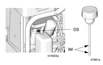
Change break-in oil in a new unit after first 250 hours of operation or within 3 months, whichever comes first. See Table 4 for recommended frequency of oil changes
