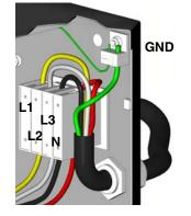
Some 3-phase models utilize a 3-phase motor. The motor must rotate counterclockwise when viewed from shaft end. To reverse rotation, disconnect power and reverse power leads L1 and L2.
