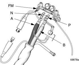
Manifold hose adapters (N, P) allow use of 1/4 in. and 3/8 in. ID fluid hoses. To use 1/2 in. (13 mm) ID fluid hoses, remove adapters from fluid manifold and install as needed to connect whip hose.  d. Connect cables (Y). Connect electrical connectors (V). Be sure cables have slack when hose bends. Wrap cable and electrical connections with electrical tape.
