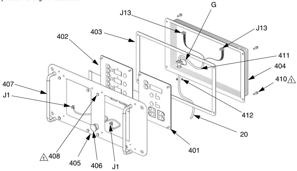
**Detail of Membrane Switches and Display Boards**
