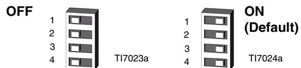
FIG. 7. DIP Switch (SW2) Settings
