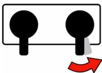
In this example, B side pressure is higher, so use the B side valve to balance pressures.
