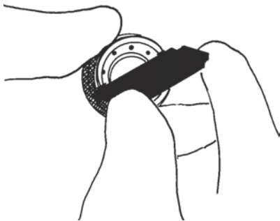
FIG. 28: Unthread Cap from PCD Body
