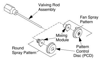
Fig. 3: Mixing Module & PCD
