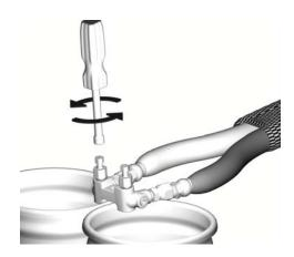
Fig. 13: Open Manual Valves
