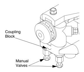
Fig. 7: Open Manual Valves
