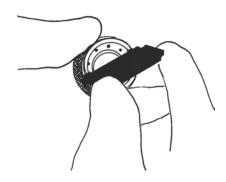
Fig. 19: Unthread Cap from PCD Body
