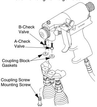
Fig. 8: Install Coupling Block
