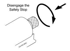
Fig. 5: Safety Stop - Disengaged
