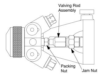
Fig. 10: Valving Rod Adjustments
