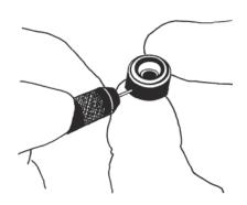
Fig. 20: Clean Module Ports
