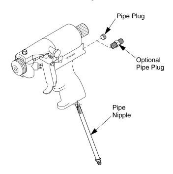
Fig. 9: Air Inlet Configuration
