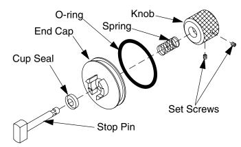
Fig. 17: End Cap/Safety Stop Assembly
