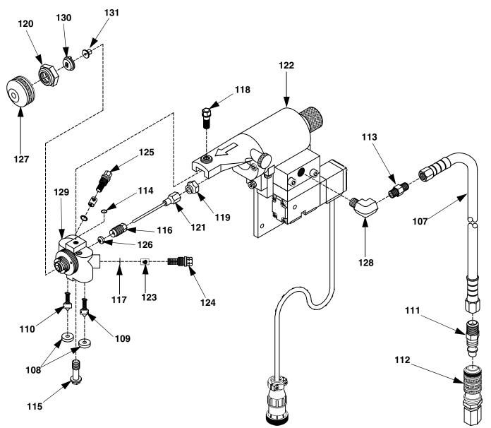
Fig. 21: GX-8P Spray Gun Final Assembly
