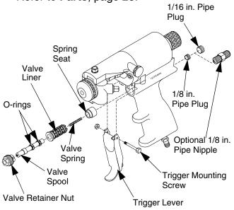
Fig. 18: Replace Trigger Valve O-Ring
