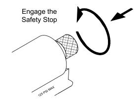
Fig. 4: Safety Stop - Engaged
