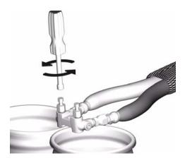
FIG. 13: Open Manual Valves
