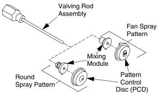
FIG. 3: Mixing Module & PCD
