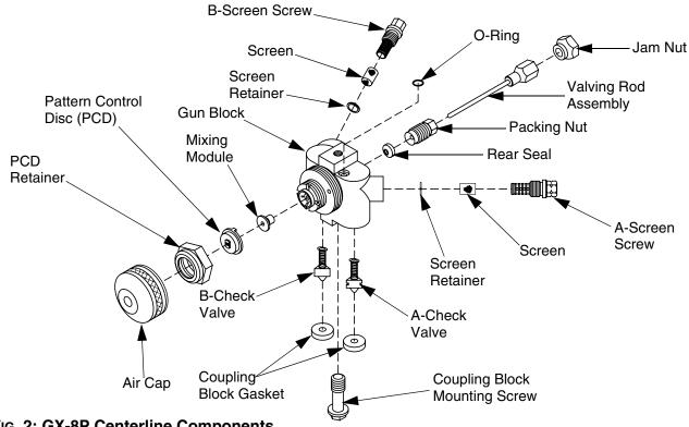
FIG. 2: GX-8P Centerline Components
