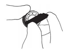
FIG. 19: Unthread Cap from PCD Body
