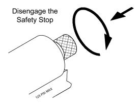
FIG. 5: Safety Stop - Disengaged
