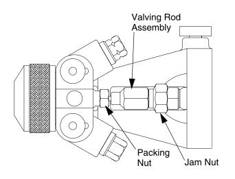
FIG. 10: Valving Rod Adjustments
