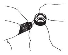
FIG. 20: Clean Module Ports
