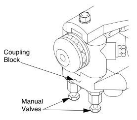
FIG. 7: Open Manual Valves
