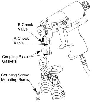
FIG. 8: Install Coupling Block
